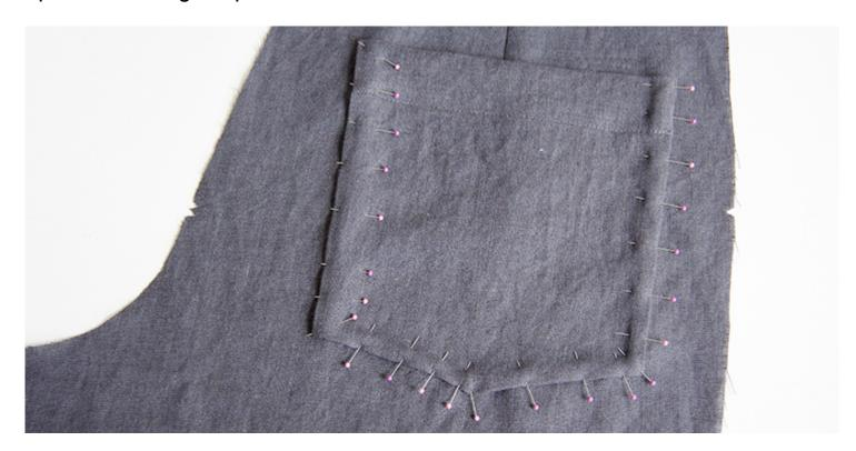
20. Topstitch the pockets in place (single or double lines) and reinforce the top corners with two small bar tacks.
